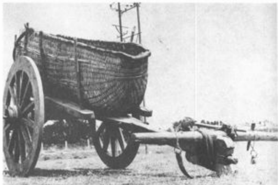
Traditional Bullock Cart with Cane Basket and Traditional Yoke System, India.
