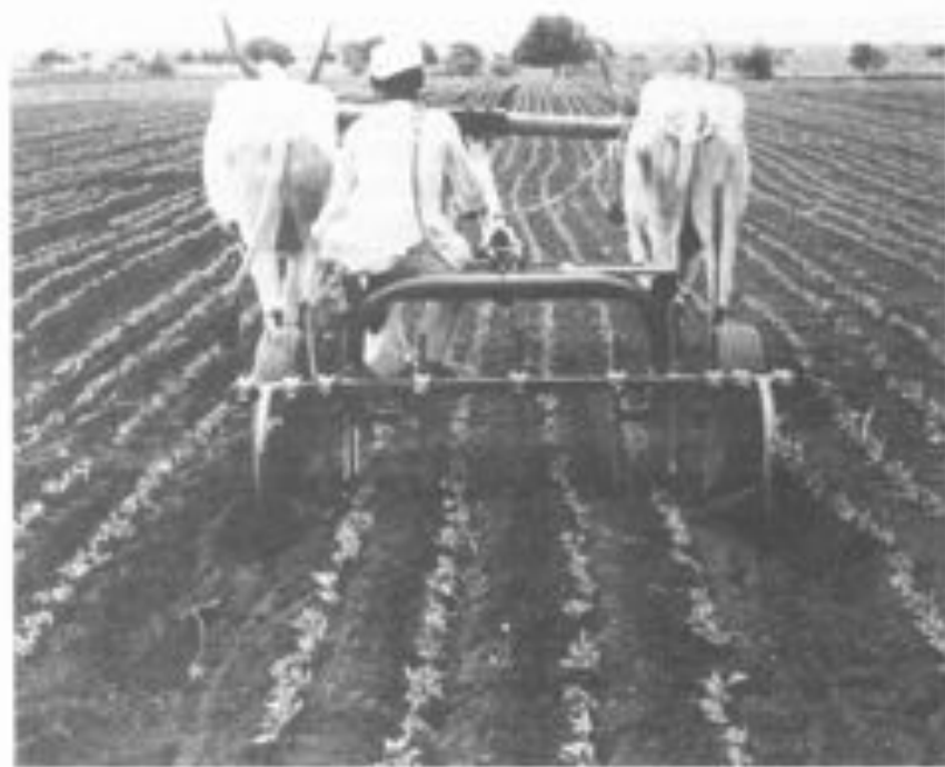
Figure 6.10 Animal Drawn Multipurpose Wheeled Tool Carrier.
