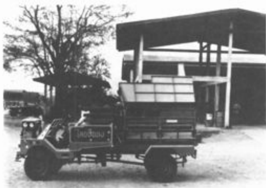
The "Iron Buffalo" Engine or Road Vehicle, Thailand.
